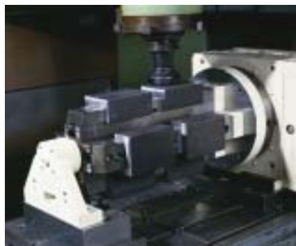
8 workpieces with 24 faces to be machined
